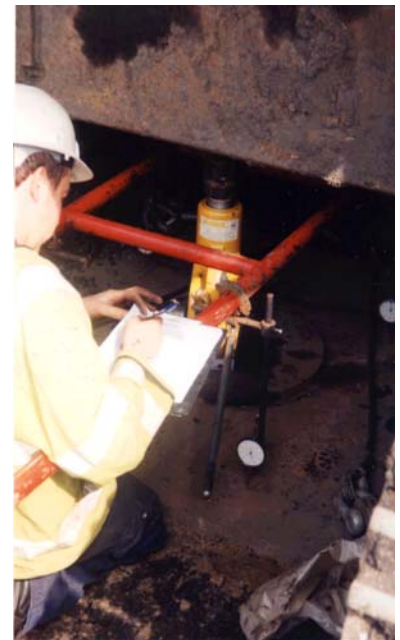
Plate Load Test being carried out
