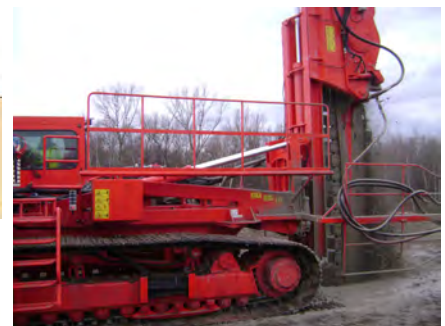
Trenchmix boom soil mixing by the dry process with powder
